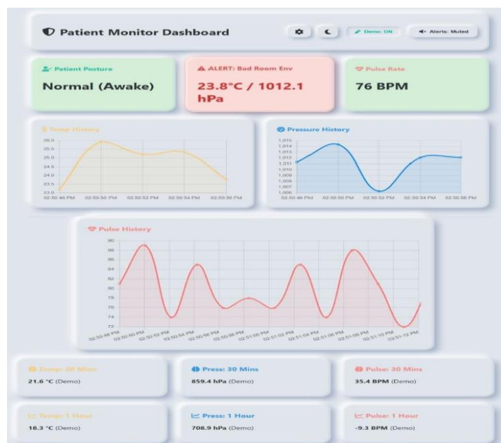
Fig.3.Web Dashboard Displaying Real-Time Patient Monitoring Data.
