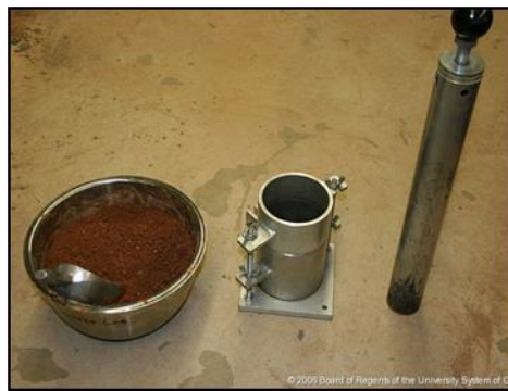
Figure 5 Compaction Test Apparatus.
