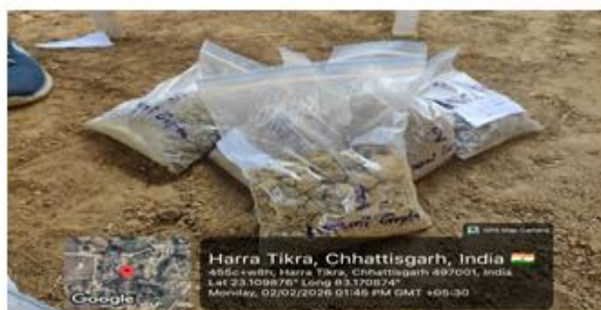
Figure 1: Polythene bags utilized for collecting and storing soil samples from the field to prevent moisture loss and cross-contamination.
