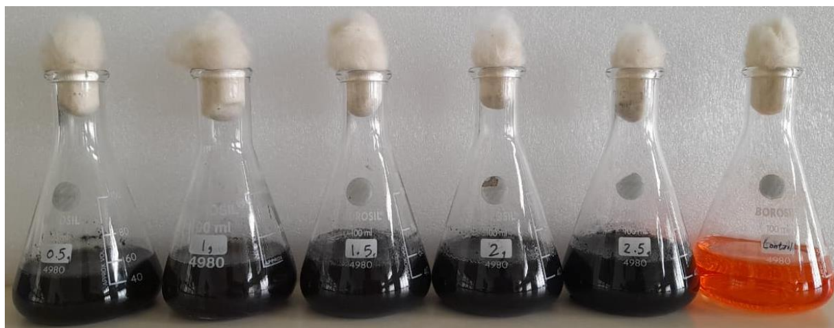
Figure 3: Dye reduction with free activated charcoal powder
