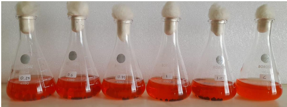
Figure 2: Dye reduction with immobilized beads
