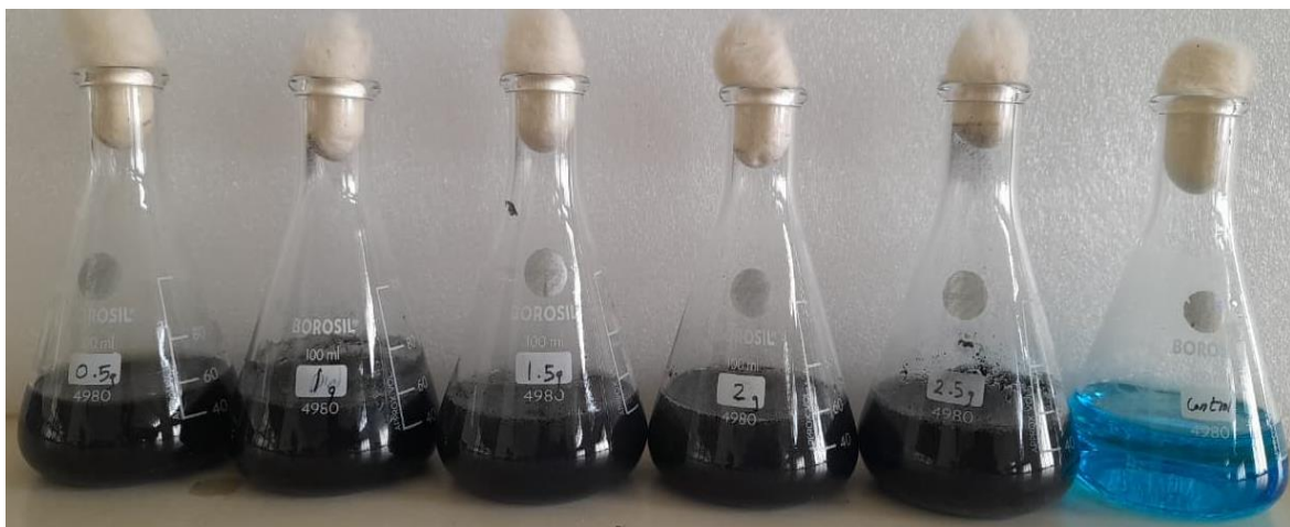
Figure 2: Dye reduction with immobilized beads
