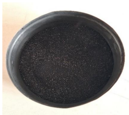
Figure 1: Activated charcoal prepared from coconut shells.
