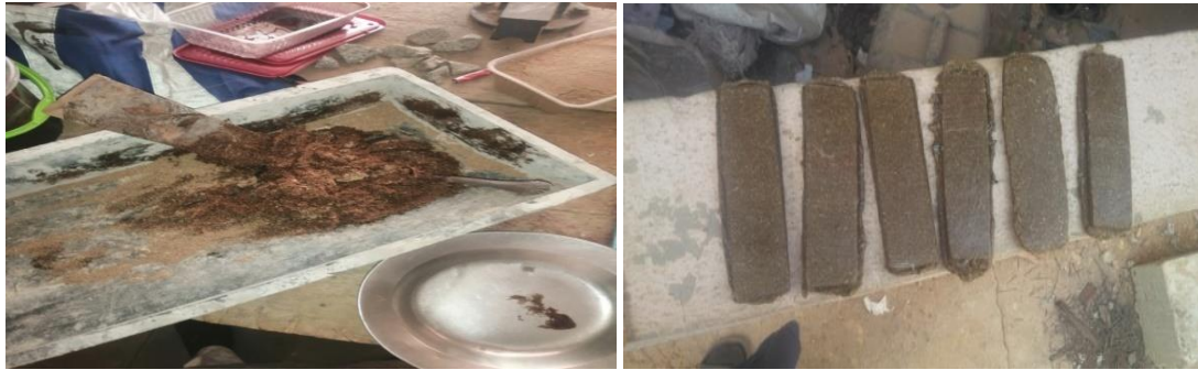
(a) Homogeneous mixture of peanut shell particleboard (b) Drying of peanut shell particleboards
