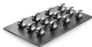
Fig 3.1 Curved C-shaped fin attached to the absorber plate
